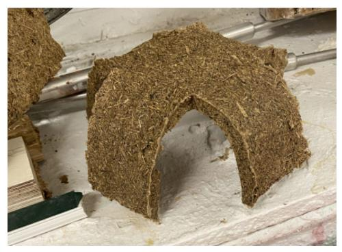
bent 1/4 scale model hide glue and ground corn husks
