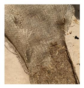
layers of jute and corn mixture are alternated in mold.
