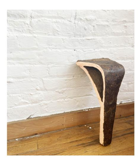
I decided to focus on a full scale sample of the leg because of cosntant rain that delayed the drying process. the sample turned out to be considerably lighter than the previous and was able to support 50lbs.
